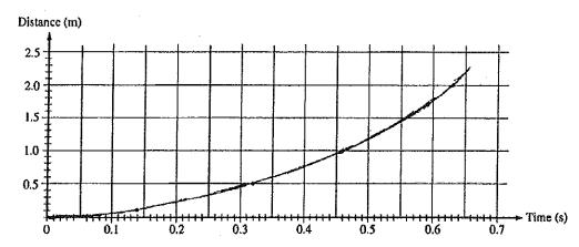
b. Distance and time are related by the equation  $D = \frac{1}{2} gt^2$ . To yield a straight line, the quantities that should be graphed are D and  $t^2$  or and t.
