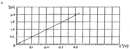
d. The slope of the graph of D vs.  $t^2$  is  $\frac{1}{2}$  g. The slope of the line shown is  $4.9 \text{ m/s}^2$  giving  $g = 9.8 \text{ m/s}^2$
